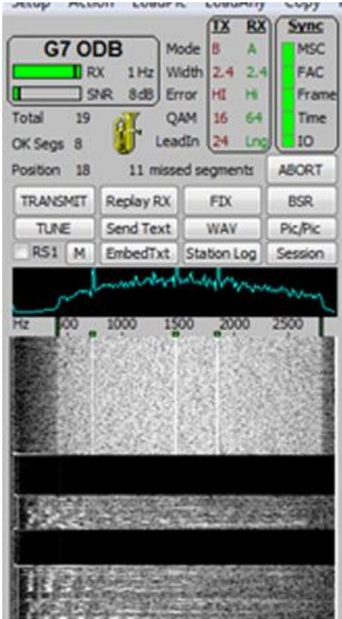
*This Picture shows an active Receive of a Transmission from G7ODB*
